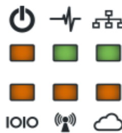
Figure: Power supply does not have redundancy
