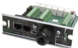
Dry contact, Management Options, Dry Contact I/O Card, monitor external UPS environmental sensors, output relays, and input contacts
